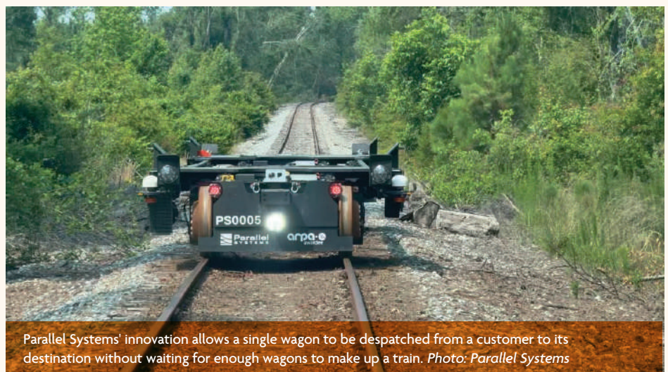
Parallel Systems have prototypes - seen here on the Association of American Railroads test track in Pueblo, Colorado - that worked and have got safety clearance from the Federal Railroad Administration for the first commercial pilot on the main line. Photos: Parallel Systems
