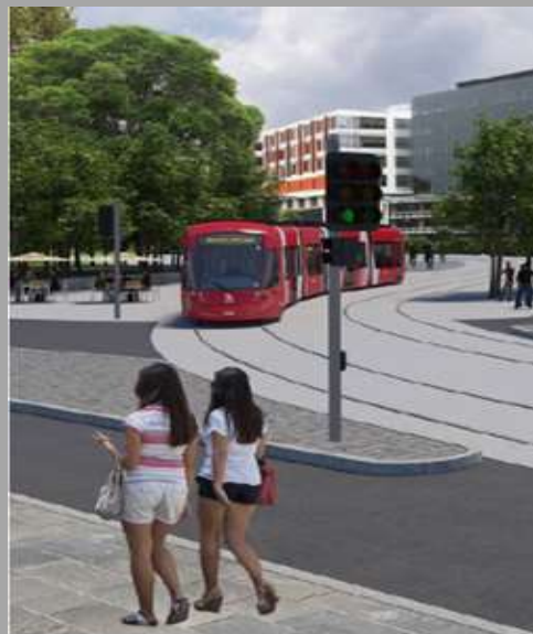
NO OVERHEADS: The city's light rail will use battery storage technology.
